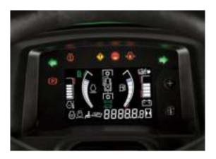
**The dashboard approach** – Electronic Fuel Gauge. Engine Temperature Gauge. Tachometer with Best Cut Target Zone. An Electric Power Take-Off (PTO) engagement indicator. All at a glance and within easy reach.
