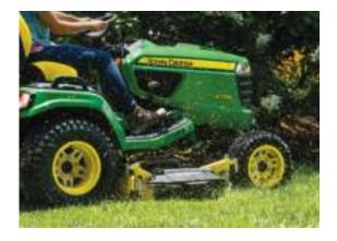
A high-capacity mower deck, solid stamped out of 9-gauge steel to handle the tall stuff.
