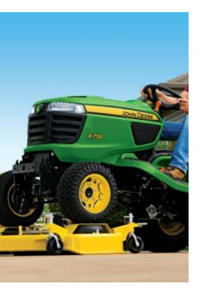
With an AutoConnect deck, attaching and removing your mower deck is easier than ever. Drive over ramps can quickly be removed, without tools, for access to mower deck.
